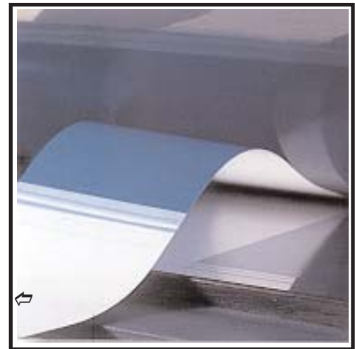
Figure A - Printed ink film splitting between the blanket and the impression block. Paper is attached to the load cell at the left (arrow)
