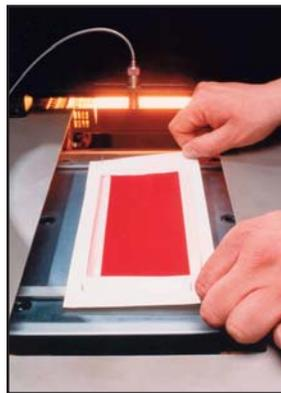
**STEP 4:** An IR sensor at the oven’s exit records the Paper Surface Temperature (PST).
