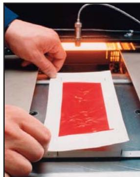
The printed sample is removed and placed on a chill color to bring the ink temperature back to ambient conditions.
