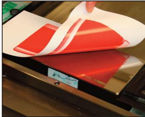
**STEP 3:** The printed sample is then heated in the “Heat Set Tester”. The paper is placed on the machine and is passed through an oven where quartz lights super-heat the sample on both sides.
