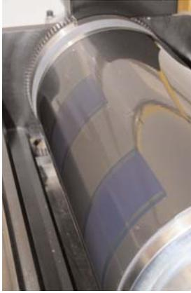
Photo showing blanket ready for the mottle test. From left to right, 4 films of ink and varnish. Film thickness of each is 0.05 mil
