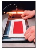
**STEP 4:** An IR sensor at the oven's exit records the Paper Surface Temperature (PST).
