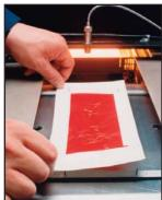
The printed sample is removed and placed on a chill color to bring the ink temperature back to ambient conditions.
