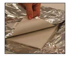
**STEP 2:** The paper sample is cut for testing and immediately printed on both sides, to simulate typical coverage on press. Here we use a special red ink, at a film thickness of 0.05 mil on both sides.
